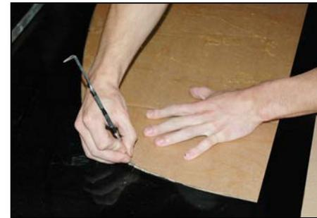
With the template in place, use a sharp object like a nail or a scribe to transfer the profile to the splitter panel. Scribe straight lines to fill the gap where you have moved the panel forward to allow for the forward projection.
