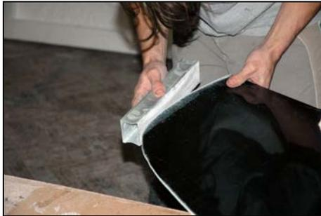
Once you've cut the panel, use a sanding block (or some 120 grit sandpaper wrapped around a block) to smooth out the cut line just up to and past the line that you scored on (to erase the line).
