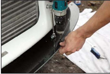
Using a 6.5mm drill bit drill through the splitter panel at the point you have marked.
