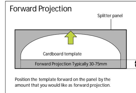
Having decided on the amount of projection you want, you should add this amount to the depth of the splitter you drew on the cardboard template by positioning the cardboard template forward on the splitter panel by this amount.
