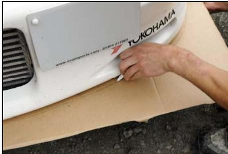
Next, use a pen to carefully draw the profile of the bumper onto the cardboard sheet. Be careful not to allow the cardboard to move, relative to the bumper during this process. Once you're done hold the template in place and check that the line follows the bumper all the way round and that the back of the cardboard still lines up with the back of the bumper.
