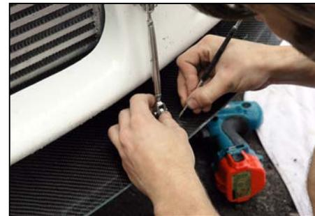
With the tops of the tie-bars in place, align the bottom half of the tie-bar with the panel and put a small mark showing this point. Ensure that both tie-bars are aligned symmetrically.
