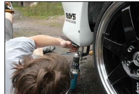
With luck you should be able to get a couple of G-clamps in place to hold the splitter panel to the bumper. If you can do this it is also helpful to support the splitter in the middle to prevent it from 'sagging' between the two clamp points.
