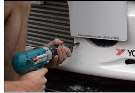
Mark the correct position for the top fastenings using a pencil. Check the alignment both vertically and horizontally to ensure the two tie bars will be symmetrical.
