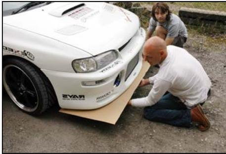
Using a large sheet of cardboard (probably some of the box that the splitter came in), position the cardboard underneath your front bumper and align it so that one edge is at the rear-most point of the front bumper/spoiler.
