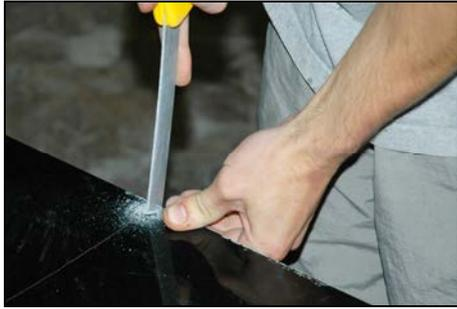
Cut the panel following the line that you scored onto it. Cut slightly outside of the line so that you can rub the cut line smooth.
