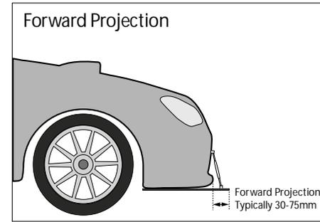
The next step is to decide how much you want the splitter panel to project forward past the front of your bumper. In most installations, this should be about 40mm but this is entirely down to your taste. Increasing this distance will increase the wind 'splitting' effect of the splitter.
