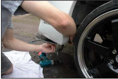
You should then use 2 of the bolts and nyloc nuts with 4 washers to fix the splitter to the panel in these two places.
