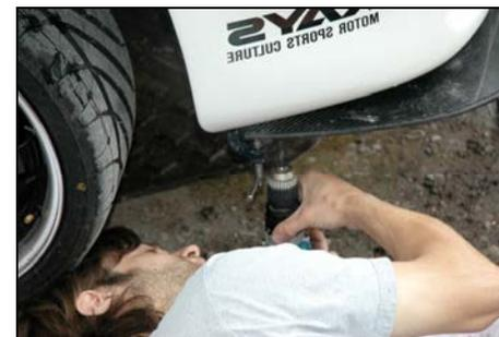
With the splitter held firmly in place, using an 8.5mm drill bit, drill through the panel and through the bumper from the underside at the rearmost point (providing the panel makes good contact with the bumper there).
