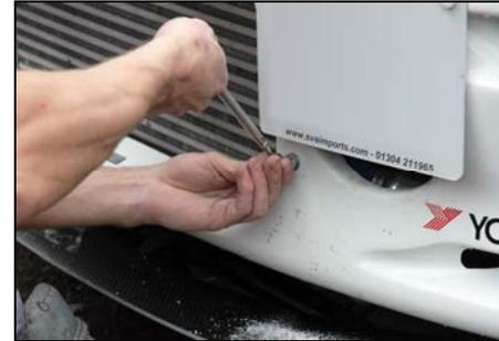
Pass an M6 bolt (with washer fitted) through from the back of the bumper and into the threaded bush at the top of the tie-bar. Tighten the fixing by turning the whole tie-bar and/or tightening the nut from the inside using a hex key.
