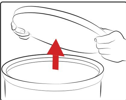
Once air can no longer be heard passing through the filter the chamber will be back to normal atmospheric pressure.
